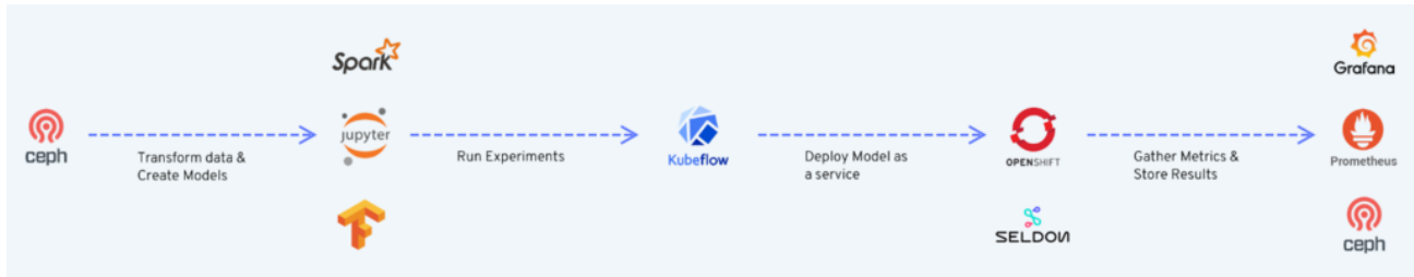
Figure 11-15: Basic pipeline for Open Data Hub
